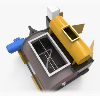
**The FoamX** mixer has a dedicated foam generation tank where the foaming agent is placed then subjected to carefully calculated amounts of water and compressed air reaching the desired foam specification.
